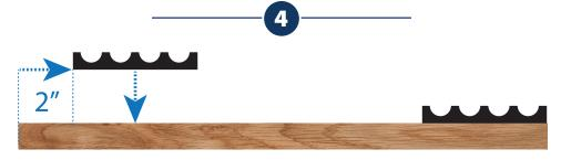
On the other end of the ripped half, measure in 2" from the end and secure one of the notched bars (1) at that mark.
