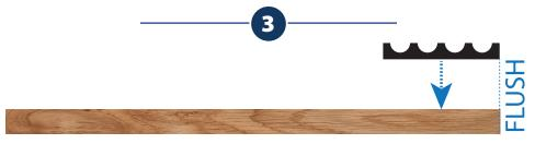
On one of the  $2'' \times 4''$  ripped halves, use the  $1\frac{1}{4}''$  Wood Screws (6) to secure one of the  $6\frac{3}{4}''$  notched bars (1) flush to one end as shown above.
